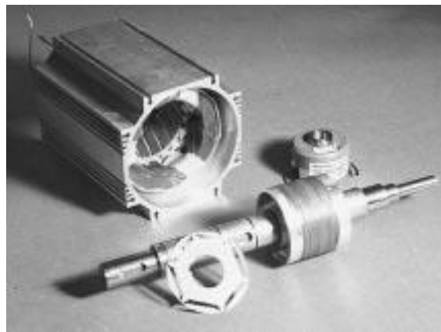
(d) Circumferential interior PM (Buried)
